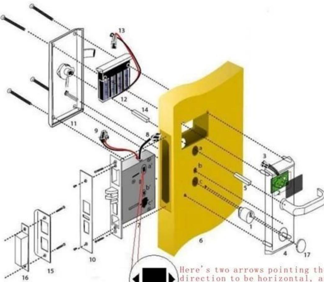
Here's two arrows pointing the direction to be horizontal, and the lock cylinder cover on the arrow on the upper, non-vertical point!
