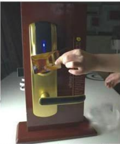
opening the door with RF card
