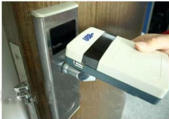
collect opening records from hotel lock
