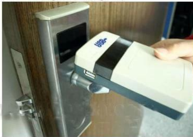
collect opening records from hotel lock
