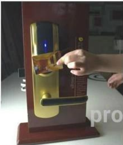
opening the door with RF card
