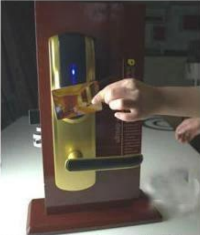
opening the door with RF card
