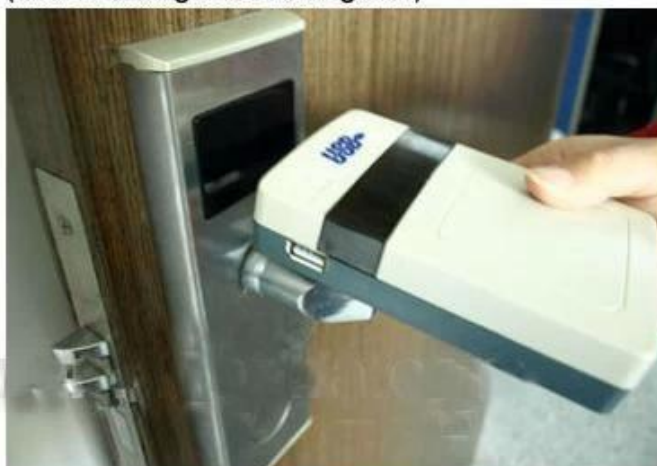
collect opening records from hotel lock
