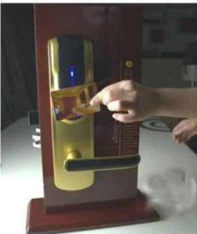
opening the door with RF card
