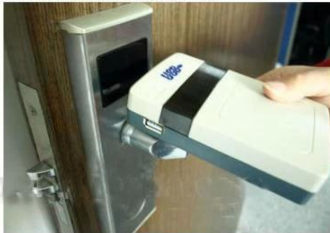
collect opening records from hotel lock
