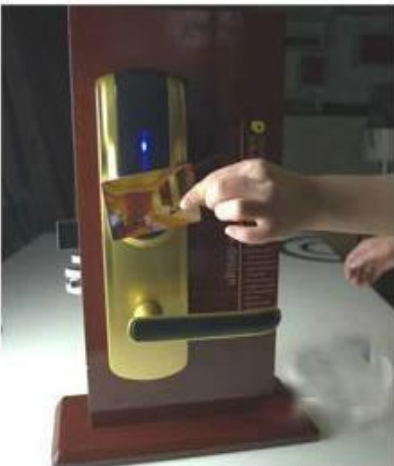
opening the door with RF card
