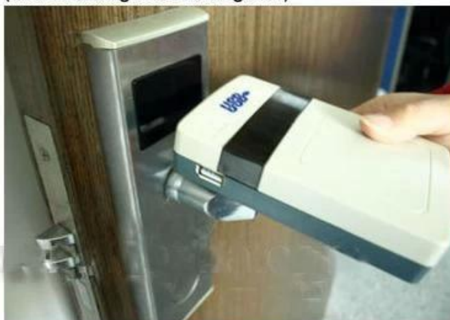
collect opening records from hotel lock
