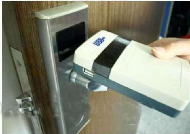
collect opening records from hotel lock
