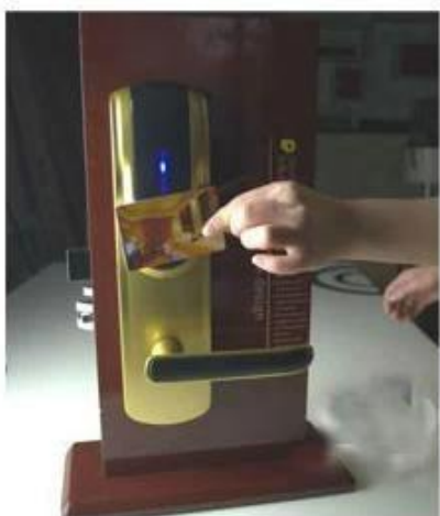
opening the door with RF card
