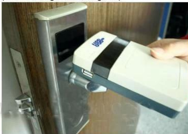
collect opening records from hotel lock
