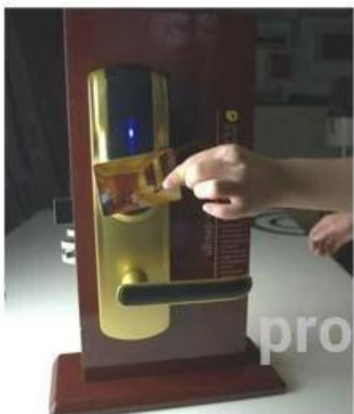
opening the door with RF card
