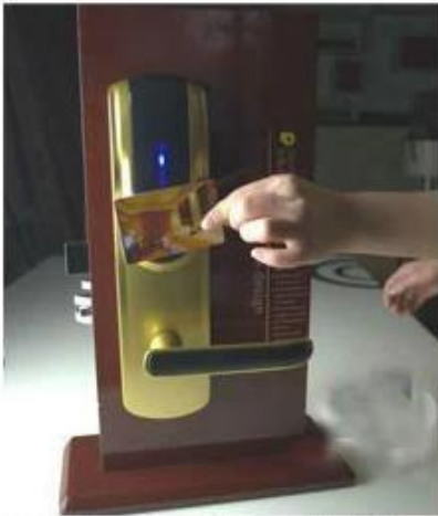
opening the door with RF card
