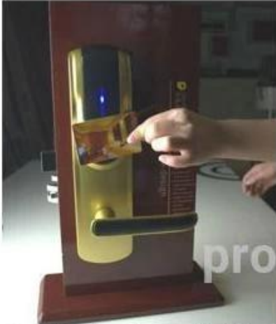
opening the door with RF card
